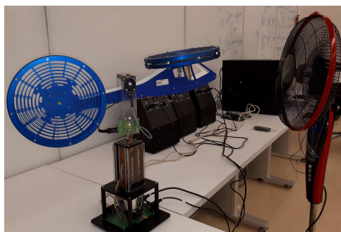
Fig. 17. Experimental setup under wind gust.
